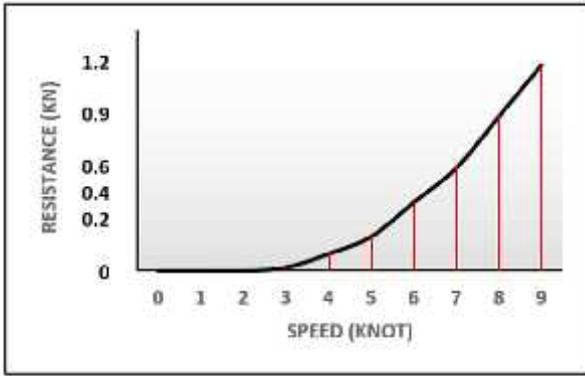
Figure 3. Graphic of Resistance vs Speed comparison
